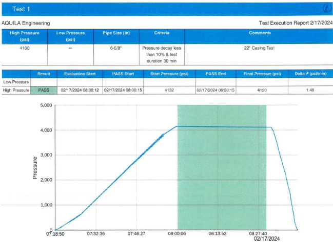
Figure 8 – Casing Integrity Pressure Test
