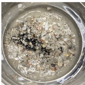
Figure 2: Slot cell after test with disk removed
