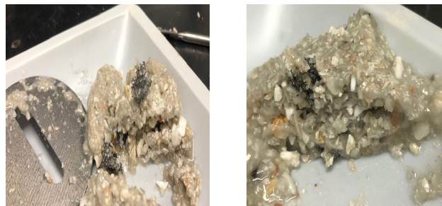
Figure 6: Filter cake pictures showing the integrity of the cake built on slot disc after the test
