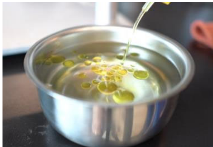
Figure 3: Dispersible lubricant floating on top of lubricity meter cup
