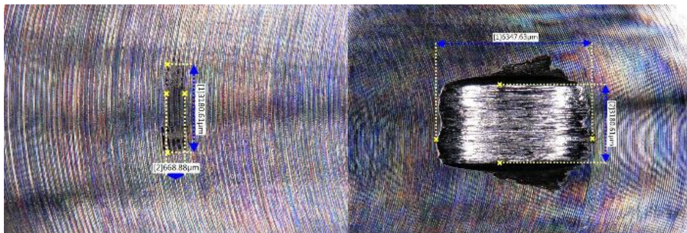
Figure 5 (left) : A high film strength lubricant shows a small scar width. Figure 6 (right): A lower film strength scar with galling.
