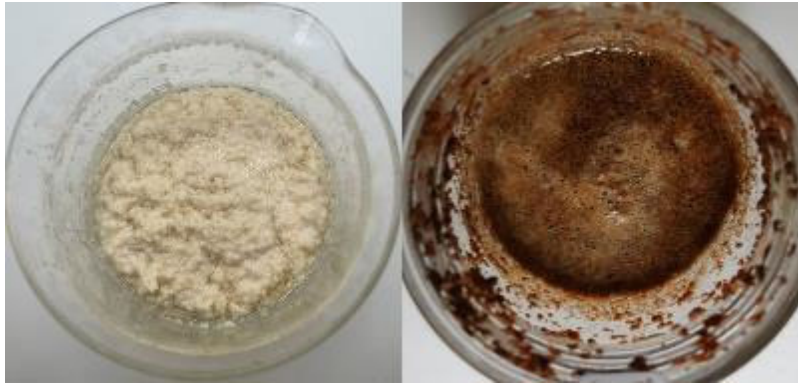
Figures 1 (left): Cheesing and Figure 2 (right): greasing from Farnum, Toomes, and Offenbacher (2023)
