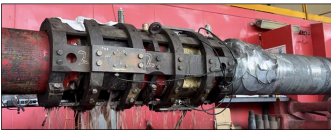
Fig. 10 – RSS in flow tester with force and pressure test cage around the steering housing. Measuring real-time pad force and pad pressure during in-house LCM threshold testing.
