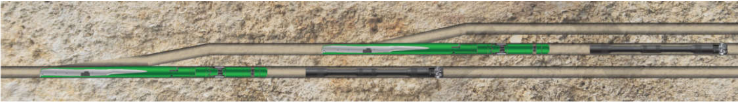
Fig 9: Image representing dual whipstocks in lateral application to sidetrack around multiple fish.
