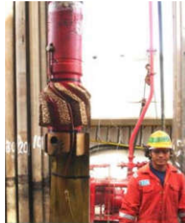
Milling BHA Made Up to Hydraulic Whipstock
