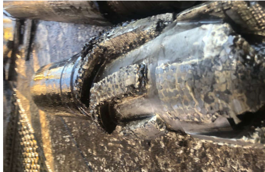
7-3/8-in OD Mill after window cut
