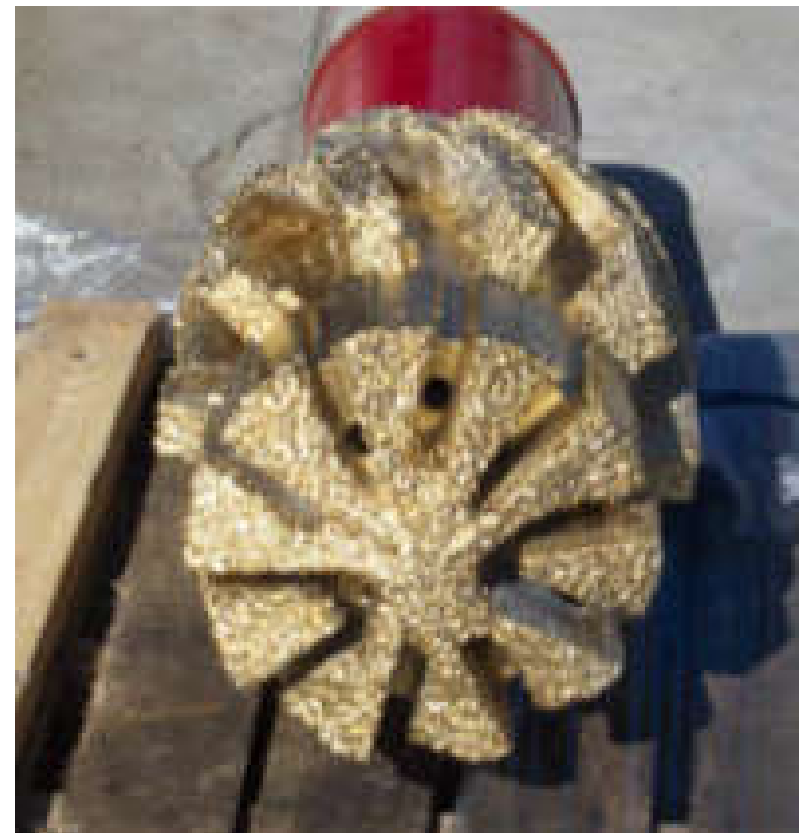
12-1/4-in OD Mill on Location for to Bypass Obstruction – Courtesy of W
