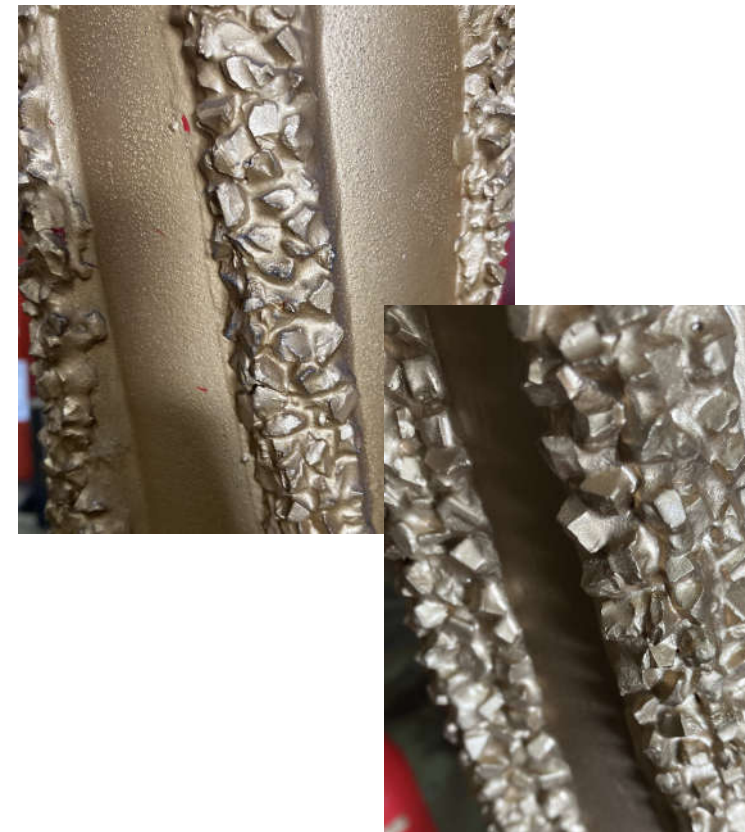
Cutting Structure Advancements - Courtesy of WFRD
