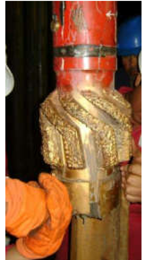
Lead Mill Made Up to Hydraulic Whipstock - Courtesy of
