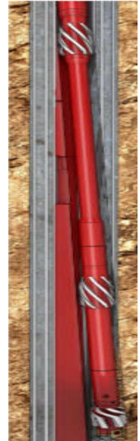
Three String Concentric Layout - Courtesy of WFL
