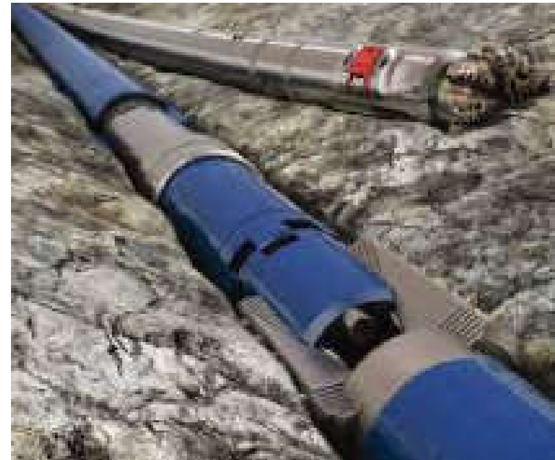
Hydraulic expandable anchored single trip whipstock - Cou
