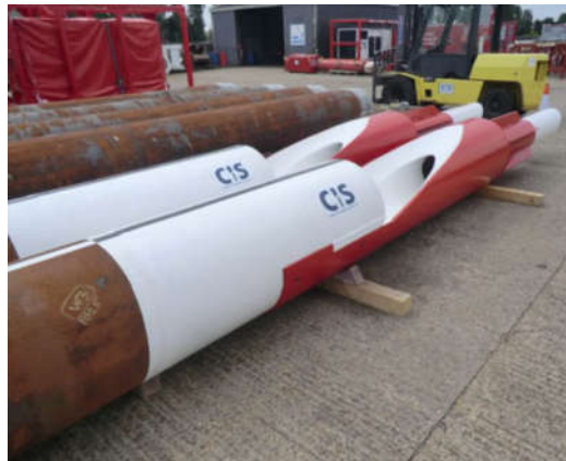
Slot recover whipstock to anchors in conductor stub - Courtesy of Acteon
