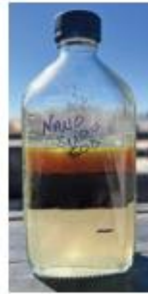
Treated sample shows clear oil, mud and water phase. Separation time was reduced from hours to ~ 5 minutes. *5 minute resting period.
