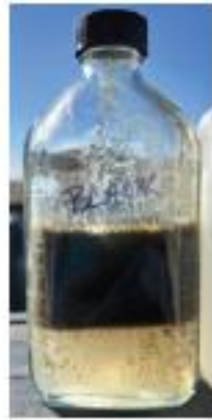
Blank sample. Very stable mix of oil, water and mud.
